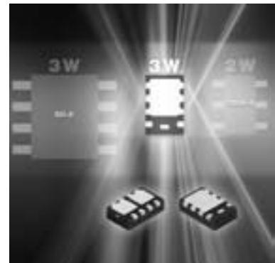
PowerPAK ChipFET provides a smaller-footprint alternative to MOSFETs in the TSOP-6 and SO-8 packages.
